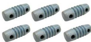
MFJ 16C06 6-pack ceramic insulators. Can be used as an end or centre insulator. These insulators will not arc over, even under full legal power. Molded ridges give extra-long voltage path to prevent high voltage breakdown. 2.5" length x 1" diameter. 1/4" holes.
