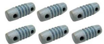
The MFJ-16C06 ceramic insulators will not arc over, even under full legal power. 2.5" length x 1" diameter. 1/4" holes.
