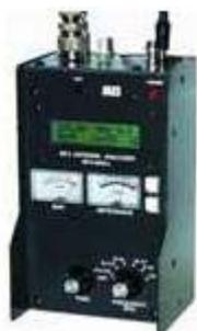
Analyze all kinds of antennas and cables. Read antenna SWR and complex impedance from 1.8 - 170 MHz and 430 - 520 MHz. Built in frequency counter.
