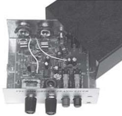
Build this inexpensive XCVR kit that really works! Includes crystal for QRP calling frequency. One Watt output. 0.3 uV sensitivity. Case not included. For intermediate kit builders.
