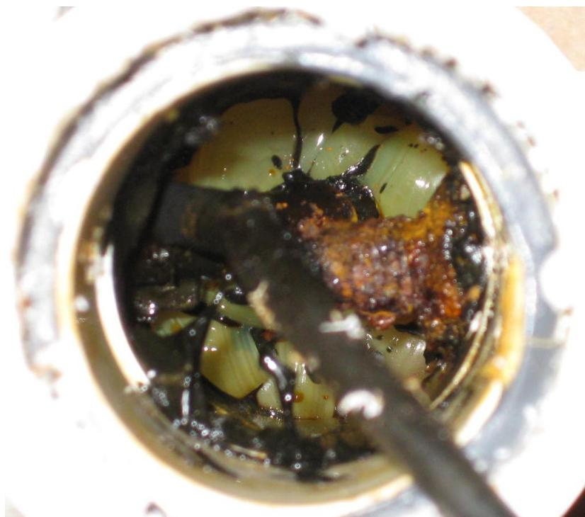
I've been told that antennas have a finite life. Sad to say, in this case it was only 5 years. The leg that wasn't loose had a silicone seal plug that required major force to extract. The end with the socket yielded water not just moisture when it was opened..... It also yielded the cause of the missed opportunity.
