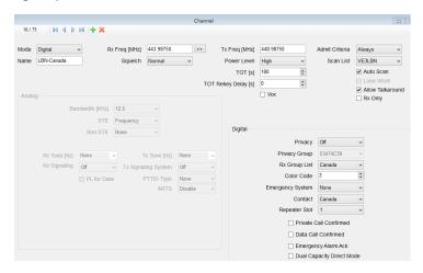
We will start at the top left corner and make our way down and across. We will not discuss the greyed out Analog section as it won't be needed for this example. Keep in mind that these are the settings for a Radioditty GD-77 handheld and other models may have the same fields but slightly different option choices.
