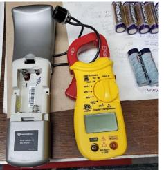
What I did was to load a good AA cell (one of the new ones) in position 1. I checked the voltage of the target 'bad' cell prior to loading. The target 'bad' cell was then loaded into position 0.
