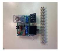
Stan VE3ILU has sent us some information on this protection circuit that he is designing for those inexpensive switching power supplies available on Amazon. It does nothing except light the green LED until tripped. I left it in the tripped mode with the red LED on for over three hours. Then powered down - and tested it again. No problems. During this week I will put it on a breadboard - with a 12V
