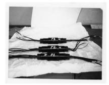
reactor building wall through a plastic assembly mounted in an air-tight box. The reactor buildings are airtight and through the ventilation system run at a slight vacuum. These assemblies were epoxy and while setting, got warm melting the coax.
