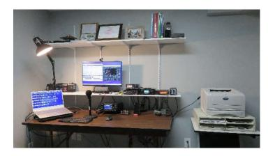
Above Shack HF Details: ICOM IC-7300 HF Rig, Heil ICM Microphone, Microphone Stand, MFJ-564 Iambic Keyer, LDG AT-200Pro II Autotuner, Diamond SX-200 SWR & Power Meter, Jetstream JTPS30LCD Power Supply and MFJ-264 1.5KW Dummy Load. VHF/UHF Details: Kenwood TM-731A 144/440 Mhz Dual Bander connected to home brew Slim-Jim antenna mounted on the rear deck.
