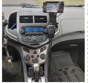
I ended up ordering an LM-500-ext heavy mount ram 1" ball mount from Lido Radio Mounts in the US. It was only \$30 and included a screw-in base, which I screwed onto the floor of the cubby hole in my dash, an arm that can be adjusted in many directions due to a ball mount on each end, and a plate for mounting the radio
