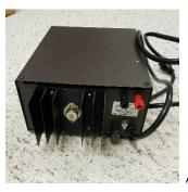
Astron RS-10A power supply. (Linear, 10
