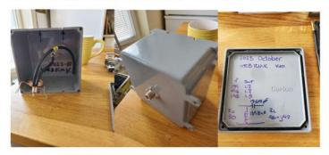
I decided to write the original measurements inside the case, so I'd be reminded if things were found to be deteriorating.
