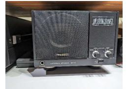
Yaesu FT1000MP MK V Field 100 watt HF Transciever 10m to 160m. the AC power supply is built in. Or you may also operate this transceiver from 13.8 VDC. This radio also features a built-in high speed automatic <u>antenna tuner</u> capable of matching loads between 16.5 and 150 ohms to better than 1.2:1 SWR. There is an <u>access door</u>
